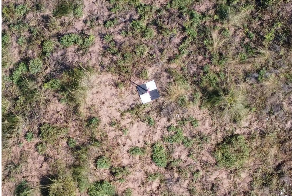
Fig. 5: Example of a ground control point using 4 x 30 cm ceramic tiles.
